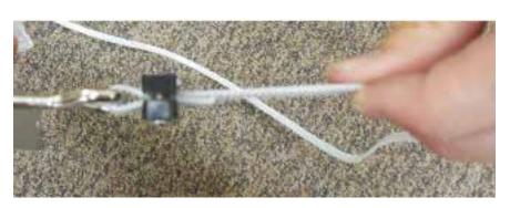
Release the belt lock lever and run the belt as shown with the teeth facing up.
