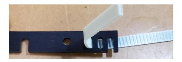
Thread the belt up the inner most slot
