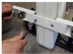
Align the two holes on the bracket to the ones on the wheel.
