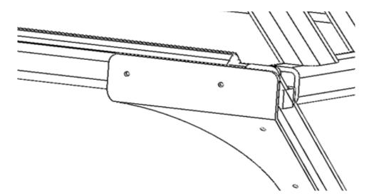
Use the same screws that were previously removed to mount the bracket to the frame.
