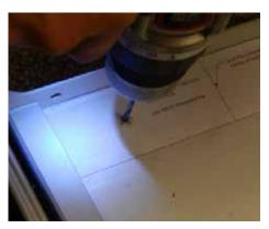
Once the hole has been drilled tap the hole using the tap size listed on the template.
