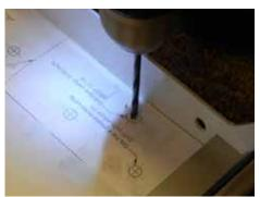
Drill the holes on the carriage using the bit sizes listed on the templates.
