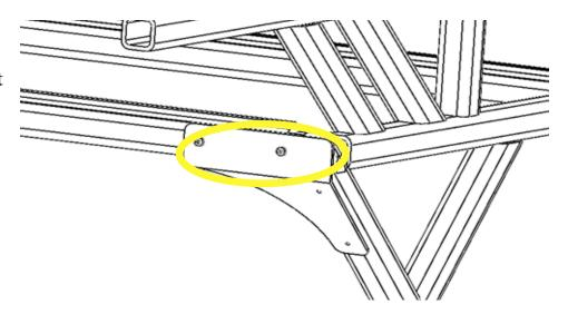
Once the screws have been removed you will go ahead and align the bracket to the frame and match the holes.
