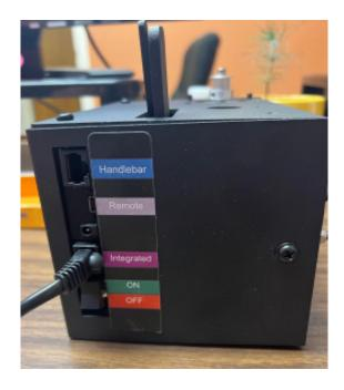
Plug remaining end of cable into the robotics port of the Perfect Stitch PCB box.
