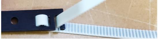
Finish by threading the belt up through the final slot
