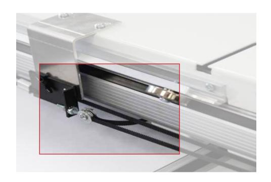
Loop the belt around the pulley on the motor box and run it back to the rear idler pulley.
