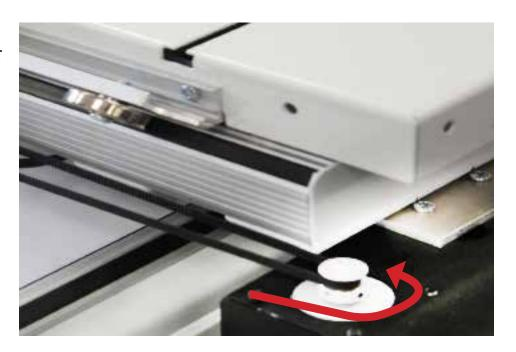
Loop the belt around the rear idler pulley and attach it to the other side of the carriage bracket with the belt clamps.
