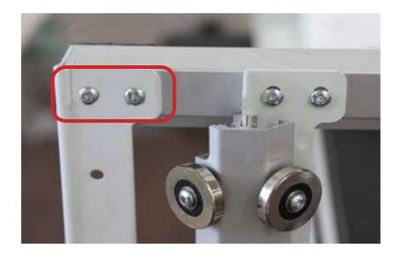
2 Use the screws removed in step one to fasten the rear idler bracket to the carriage.
