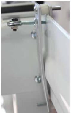
3 Use the belt clamps to attach the belt to an eye bolt.
