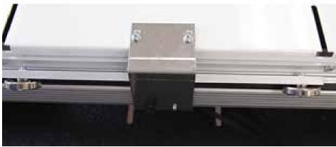
Attach one end of the black belt to the eye bolt on the carriage bracket with the belt clamps.
