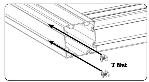
Attach Belt Bracket to T-nuts and tighten securely using provided screws.
