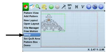
Power on the display, go to Setup > Advanced and set the machine type to Default.
