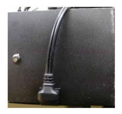
Run the cable along the carriage to the back of the machine, and then plug into the outlet or power source.
