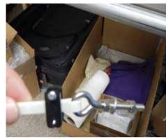
Attach the eybolts to each side of the frame in the drilled holes with the belt teeth facing up.
