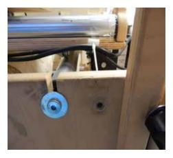
Attach the white belt to each of the eyebolts with the belt clamps.
