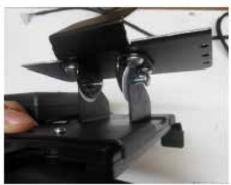
2 Loosen the faceplate screws and slide the display bracket tab into the gap.
