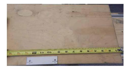
Line up the right side of the template 9 inches from the front of the carriage on the left hand side of the carriage (from front).
