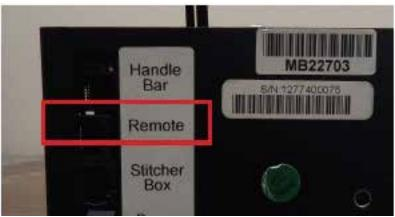
Run the cable with the handlebar cable around the back of the machine up to the display.
