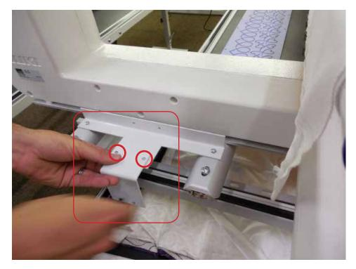
Using a Phillips screwdriver, attach the bracket with the two provided screws.
