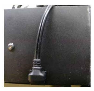
Run the power cable along the carriage to the back of the machine, make sure that the cable is out of the way of moving parts then plug it in to the power source.
