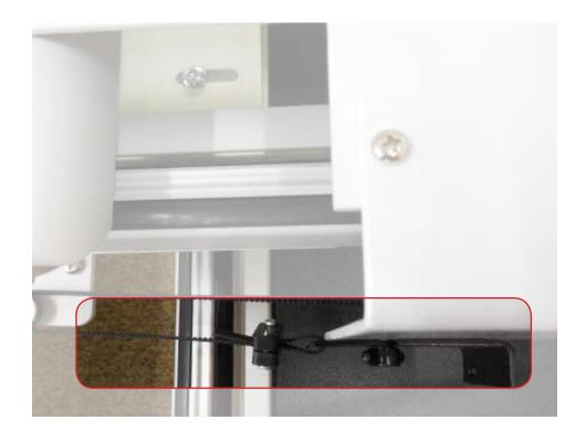
Run the belt around the rear idler pulley Making sure the teeth on the belt line up with the teeth on the pulley.
