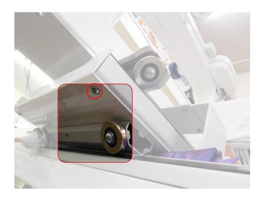
Using a hex key, remove the bolt.
