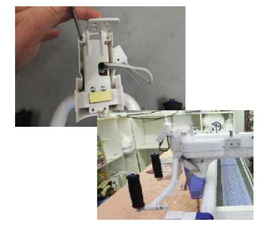
Run the handlebar wire from the handlebars along the left side of the machine, around the back and along the carriage.
