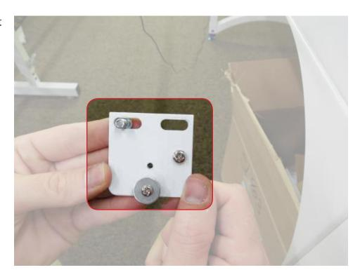
Using the hex key, reattach the bolt and idle bracket with the pulley facing up.
