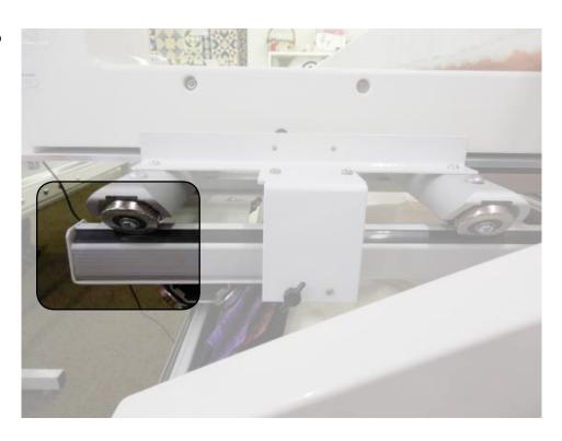
Locate this bolt on the underside of the carriage.
