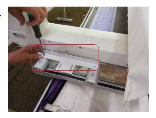
Position the secondary carriage bracket so that the left and right holes align with those on the carriage bracket and the adjustment knob is closest to the floor.
