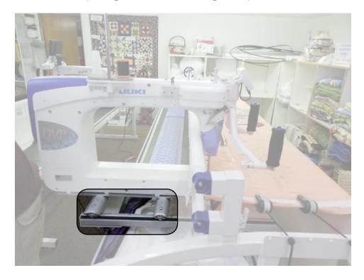
Position the carriage bracket on the carriage so that the left and right holes align with those on the carriage.
