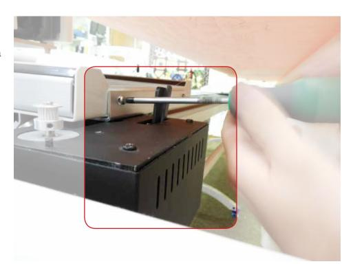
To ensure proper spacing, first attach the right screw and then the left screw.
