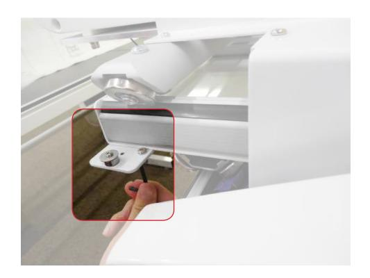
Ensure the bolt is attached in the farthest right position in the left slot of the idle bracket slot.
