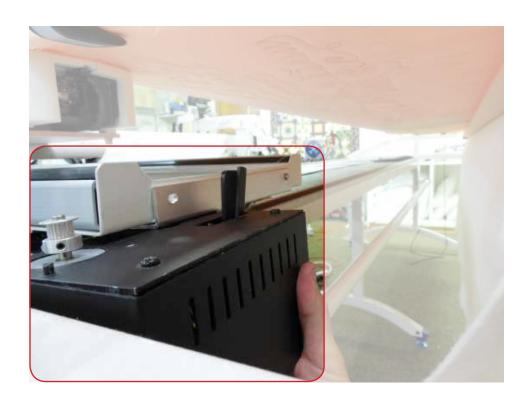
Using a Phillips screwdriver and the provided screws, attach the motor box bracket to the carriage.
