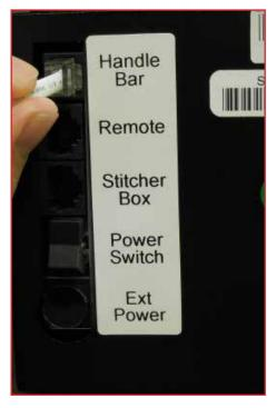
Note: It is possible to attach the handlebar wire to the rear handlebars, but Juki machines can only operate the handlebars with the Juki display connected to them. If the handlebar cable is connected to the rear handlebars, then in order to use the robot the Juki display must be connected to the rear handlebars as well.
