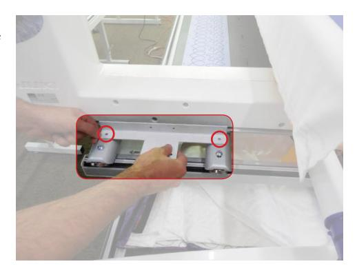
Using a Phillip's screwdriver, attach the bracket with the two provided screws.
