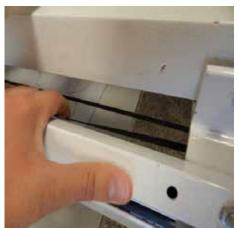
To tighten the belts use the nuts on the eye bolts.
