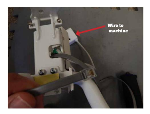
Reinsert the screws to put the cover back on the handlebars.
