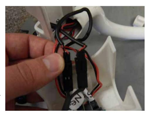
Run the side of the handlebar cable with the RJ12 (like a telephone) connector through the gap in the handlebars with the wire that the plugs the handlebars into the machine.
