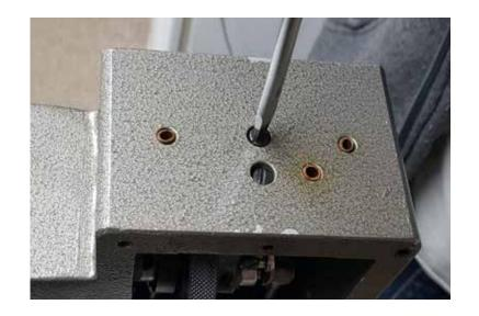
2 Slide one side of the bracket under the removed screw and replace it with the provided M4 x 20 screw and washer.
