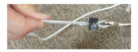
Adjust tension as needed. The belt should have about 1/2" of play with the motor box in the middle of the frame.
