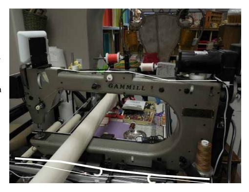
2 Use a zip ties and anchor bases to hold cables in place on the top of the machine and the side of the carriage.
