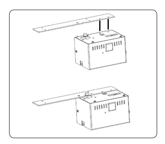
Use provided screws to attach Motor
