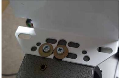
Attach the standard display to the bracket with the provided M6 x 8mm screws.
