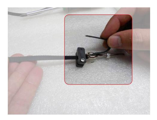
Align the belt teeth, then finish tightening the clamps.
