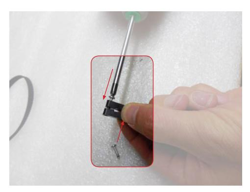
Thread the belt between the clamps, loop it around and reinsert it between the clamps.
