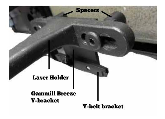
Use a belt clamp to attach the black belt to the Y-belt bracket with the teeth facing away from the machine.
