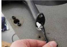
Connect the two ends of the included QuiltEZ button cable into the metal spades of the button.
