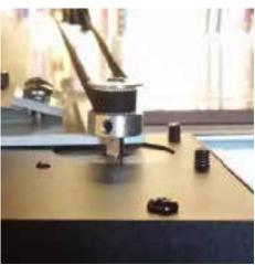
Attach the end of the belt to the other side of the Y-belt bracket.
