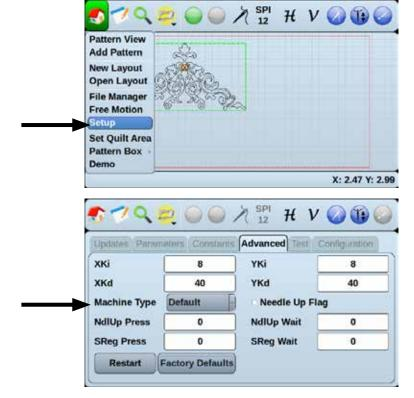
Go to the **Advanced** tab and set the machine type to Gammill.
