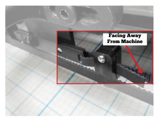
Loop black belt around the rear idler pulley and up around the top pulley on the motor box with the teeth facing in.
