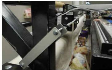
3 Use the belt clamps to attach the belt to an eye bolt.
