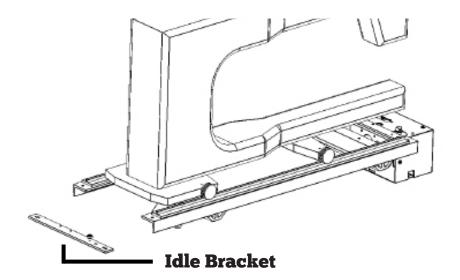
You will attach the Rear Idler Bracket to the back end of the carriage using (2) 1/4-20 x 1" screws that are provided.
