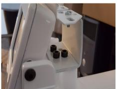
2 Use the (3) M6 x 60 mm Screws that are provided to attach the display and Handle bar to the machine.
