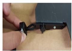
Once the belt has been attached to the carriage bracket bring the belt up and wrap it around the Motor box pulley, make sure that the belt wraps around in a **counter clockwise rotation.**
