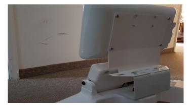
Plug the display wire into the display cable port and the other end into the remote port on the black motor box.
