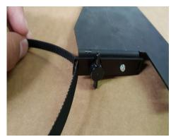
Slide one end of the belt through the slit on the belt bracket, pull it through and tighten it down using the belt brackets that are provided.
