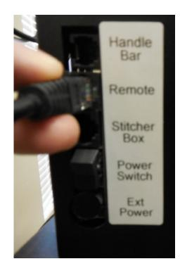
Plug one end of the handle bar wires into the handle bar port on the black motor box.
