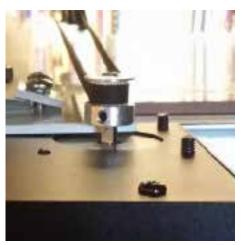
Attach the end of the belt to the other side of the Y-belt bracket.
