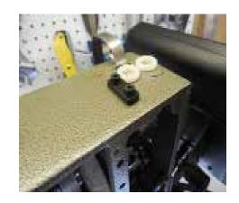
2 Slide one side of the bracket over the removed screw hole and Reinstall the removed screw
