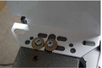
Attach the standard display to the bracket with the provided M6 x 8mm screws.
