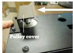
Tighten nuts onto top of screws to secure the Pulley cover.
