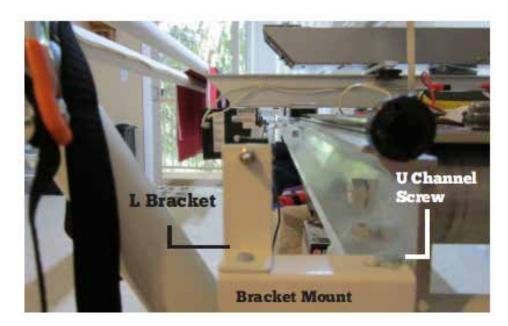
Attach the eye bolt to the top hole on the L-bracket
