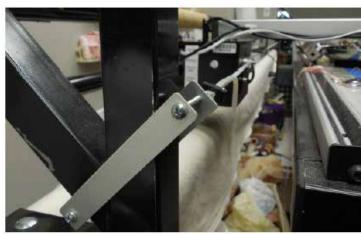
Use the belt clamps to attach the belt to an eye bolt.
