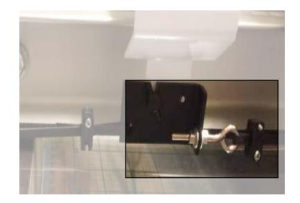
Adjust tension as needed. The belt should have about 1/4" of play.
