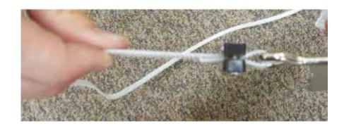
Adjust tension as needed. The belt should have about 1/2" of play with the motor box in the middle of the frame.
