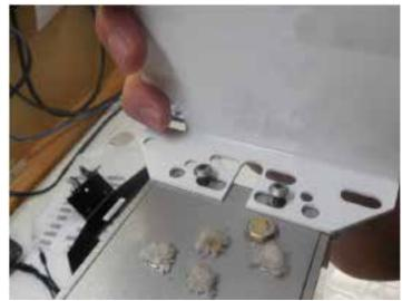
Attach the display holder to the remote bases on the display bracket with the poly disc in between.
