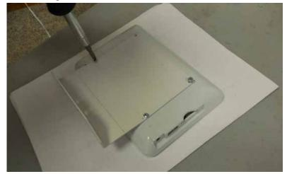
Remove the two screws on the top front of the machine.
