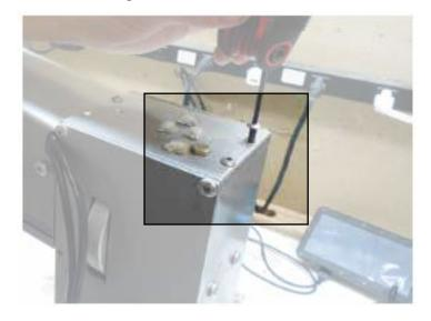
2 Use the removed screws to attach the display bracket to the machine as pictured.
