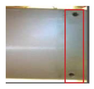
2 Use the provided screws to attach the carriage bracket to the holes on the bottom of the machine.
