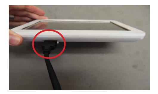
Run the display cable as pictured using he provided adhesive anchors and zip-ties.
