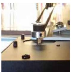
Use another belt clamp to attach the belt to the eye bolt on the carriage bracket.
