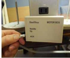
Plug one end of the network style cable into the Motor Box port on the stitcher box.
