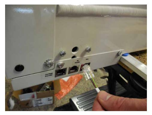
Run the handlebar cable to black motor box along side the display cable.
