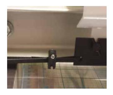
Loop the belt around the rear idler pulley and up around the pulley on the motor box. Make sure the teeth are facing in.
