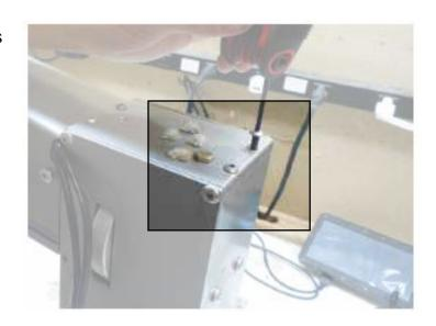
3 Use the removed screws to attach the display bracket to the machine as pictured.
