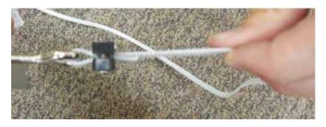
Release the belt lock lever and run the belt as shown with the teeth facing up.
