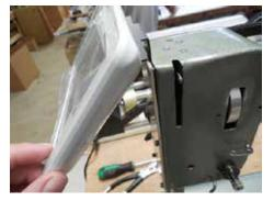
Plug the display wire into the remote port.
