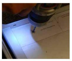
B Once the hole has been drilled tap the hole using the tap size listed on the template.
