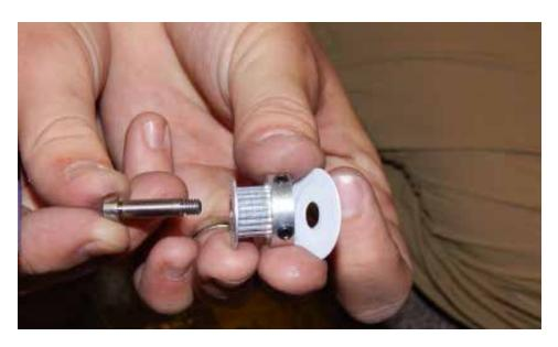
Insert the assembled pulley into the drilled hole on the carriage, and use a hex key to fasten it into place.
