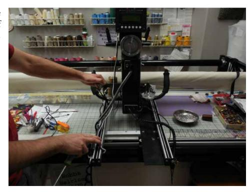
Align bracket holes with those on the back of carriage. Screw into place with provided screws.
