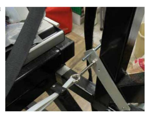
Ensure that the white belt aligns with the pulley on the black motor box, teeth facing up toward the ceiling.
